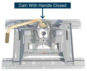
We designed our jaws and handle to work with a cam mechanism. When the handle is pinned closed, the cam keeps the jaws from opening.
