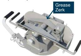
Spread a thin layer of multi-purpose grease around the inside surface of the jaws where they grasp the kingpin. You may also want to apply some grease to the kingpin on your trailer.
