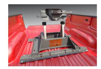
Place the coupler over the pivot arms and allow the saddle latches to fall back to their original positions. (The saddle handles should be parallel with the base in the latched position).
