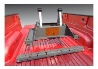
Lubricate the polyurethane bushings on top of the pivot arms with high grade lithium grease (available at your local hardware/automotive store). Pick up the coupler by lifting up on both saddle handles which will open the saddle latches.
