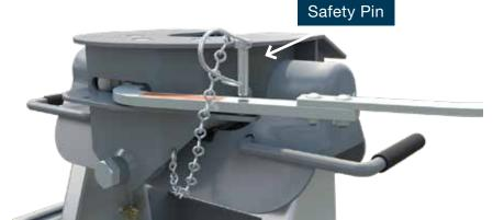
Use the safety pin to lock the handle in the open position and when you are sure that the landing gear will support the trailer, move the truck forward to release the jaws from the kingpin.
